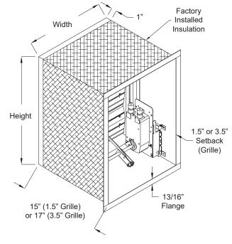
Combination Fire/Smoke Damper ▲ 1½ Hr. Rated ▲ Airfoil Blades ▲ Leakage Class II ▲ 250°F or 350°F Rated ▲ Out-of-Barrier ▲ Galvanized Steel
